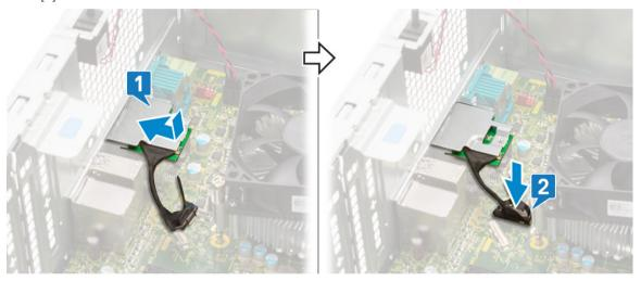
Replace the two (M3X3) screws to secure the optional VGA module to the system.
