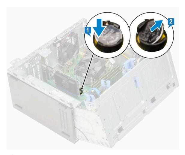
(i) NOTE: Removing the coin cell battery may reset the system board BIOS/Settings
