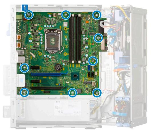
b Slide and lift the system board away from the computer [1, 2].
